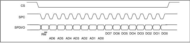
The SPI Read command consists is performed with 16 clocks pulses:
