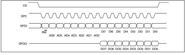
CS is the Serial Port Enable and it is controlled by the SPI master. It goes low at the start of the transmission and goes back high at the end. SPC is the Serial Port Clock and it is controlled by the SPI master. It is stopped high when CS is high (no transmission). SPDI and SPDO are respectively the Serial Port Data Input and Output. Those lines are driven at the falling edge of SPC and should be captured at the rising edge of SPC.
