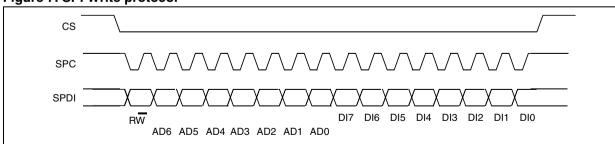
The SPI Write command consists is performed with 16 clocks pulses.
