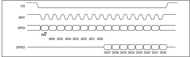
The SPI Read command consists is performed with 16 clocks pulses:
