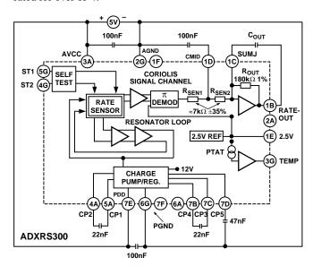
Figure 5. Block Diagram with External Components
