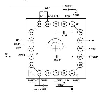
NOTE THAT INNER ROWS/COLUMNS OF PINS HAVE BEEN OMITTED FOR CLARITY BUT SHOULD BE CONNECTED IN THE APPLICATION.
