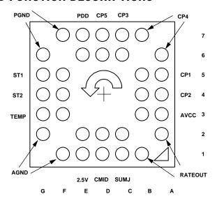
Figure 3. 32-Lead BGA (Bottom View)
